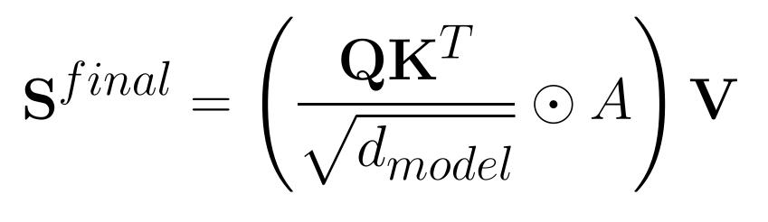
Project span representation into **Q**, K, V and perform attention (using the adjacency matrix as mask)
